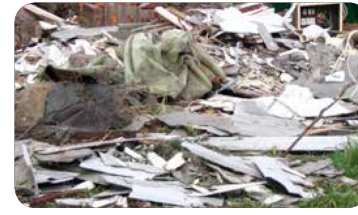
Broken asbestos cement materials from a demolition
